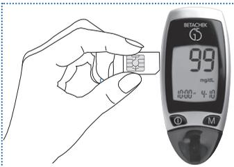
Each pack of test strips comes with a memory card that must be inserted into the meter before any tests are performed.
